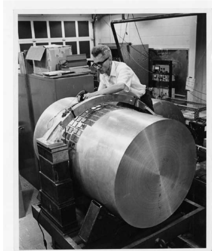
Joseph Weber (“O”) working on a resonant-mass gravitational wave antenna, or “Weber bar” (c. 1965)
