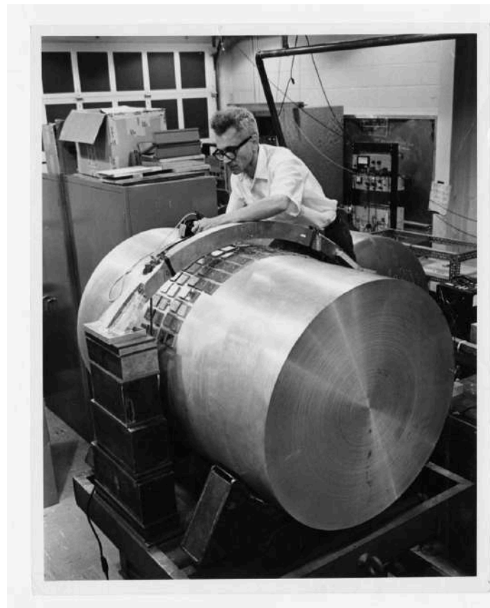
Joseph Weber (“O”) working on a resonant-mass gravitational wave antenna, or “Weber bar” (c. 1965)
